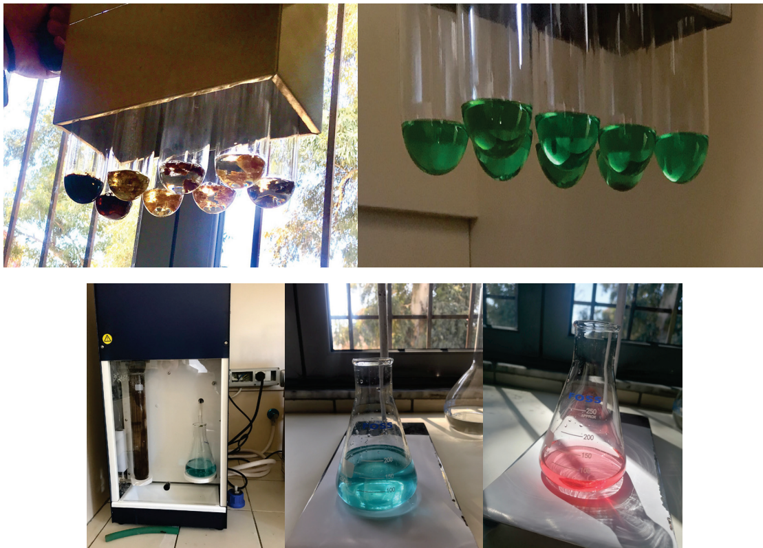
Figure 10: Total protein determined by Kjeldahl method
