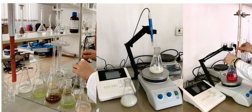
Figure 14: Total acidity determined with potentiometric method
