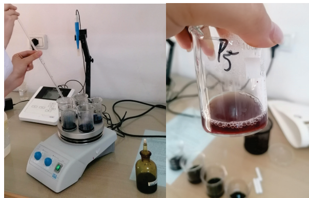
Figure 12: Sugars determined with the Lane & Eynon volumetric method
