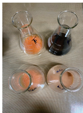
Figure 16: Samples titrated with standard silver nitrate solution 0,1N till red-brown endpoint
